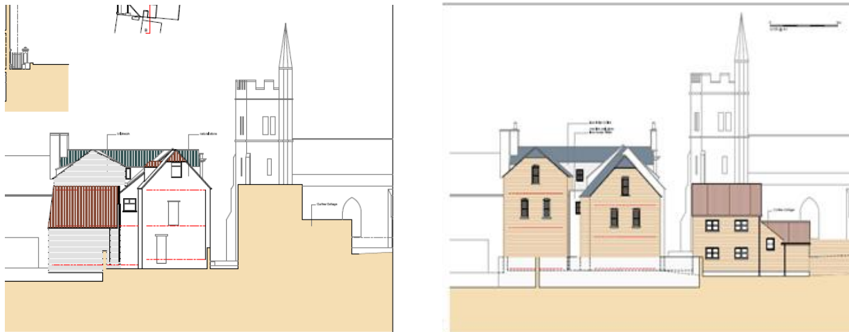
Existing (above left) and Proposed (above right) plans of South elevation and sections (Main Building)
